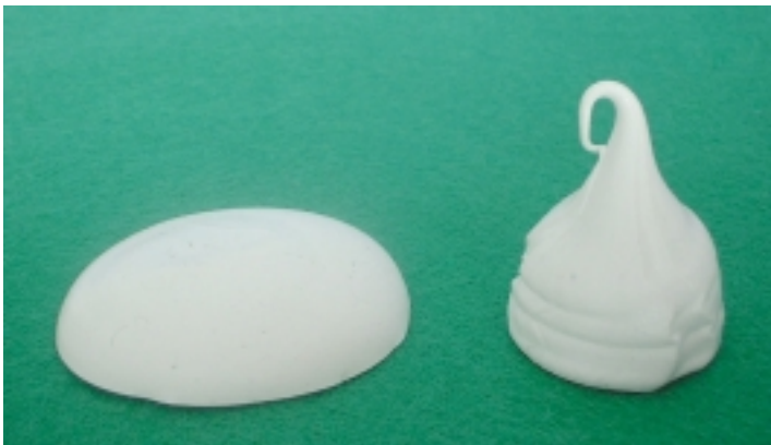
Figure 1: Cured one-component methoxysilane sealants. The sealant on the left contains no rheology modifier while that on the right was prepared using 3.5% CRAYVALLAC SL
